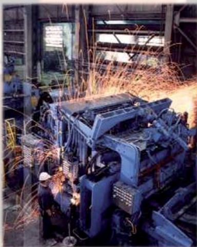
Above: Flash Butt Welder At Right: TwinLap Welder - AHSS Processing Line
