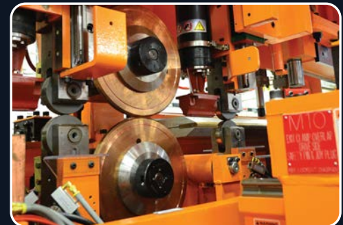
Single Pair HD Welding Heads With Hydraulic Nut and Two Pairs Planish Wheels For Single or Dual Pass Welding
