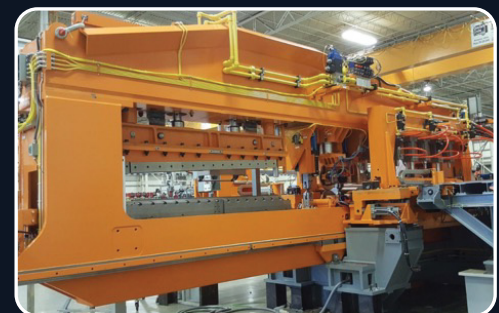
Sequence Entry Side - Movable Carriage In Post Weld Position
